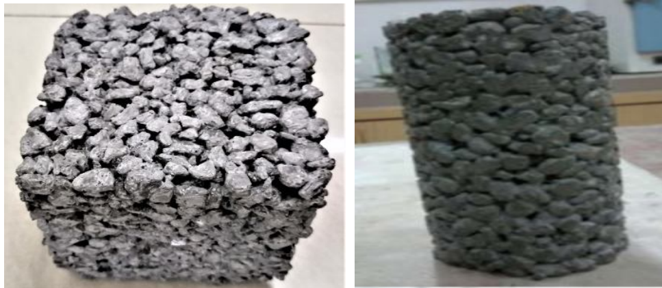
Fig 1: Sample specimens of cubes and cylinder
