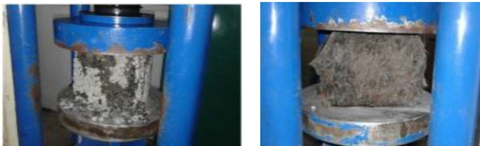
Figure 2: Cubes with fiber and without fiber
