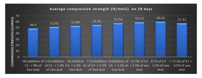
With increase in the percentage replacement of silica fume + saw dust, compressive strength also increased and the maximum value of compressive strength (peak value) was observed at 15% for 7 days whereas for 28 day highest strength was also observed at 15%. After adding more silica fume & saw dust into mix its strength starts decreasing.
