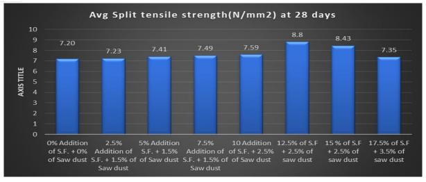
With increase in the percentage replacement of silica fume with cement + saw dust with sand, split tensile strength also increased and the maximum value was observed at 12.5%
