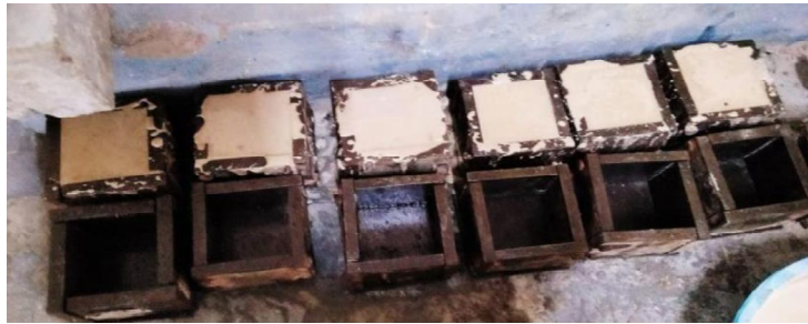
Figure 6: MOC cement mortar specimens.
