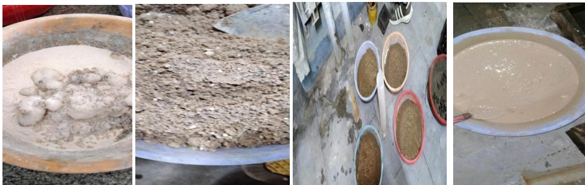
Figure 5: Sequential mixing of mortar materials
