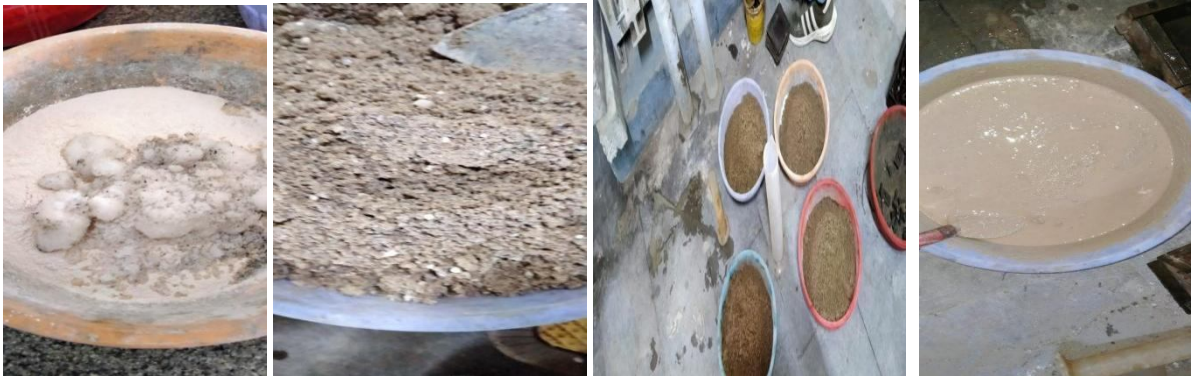
Figure 5: Sequential mixing of mortar materials
