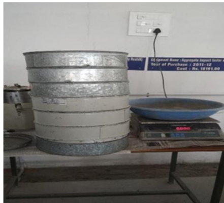
Figure 3. Gradation of coarse aggregate
