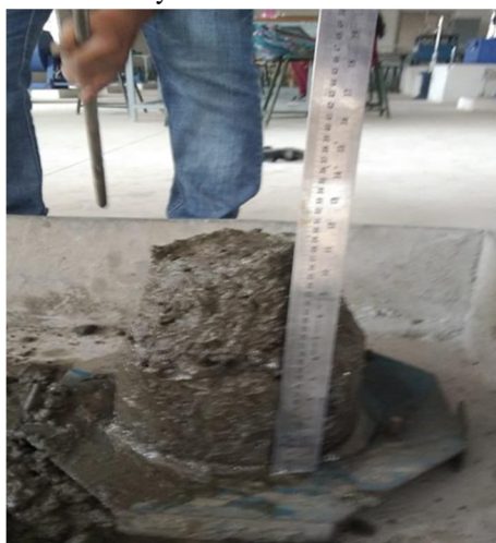
Figure 6. Slump cone test
