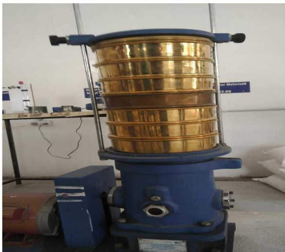
Figure 2. Gradation of fine aggregate
