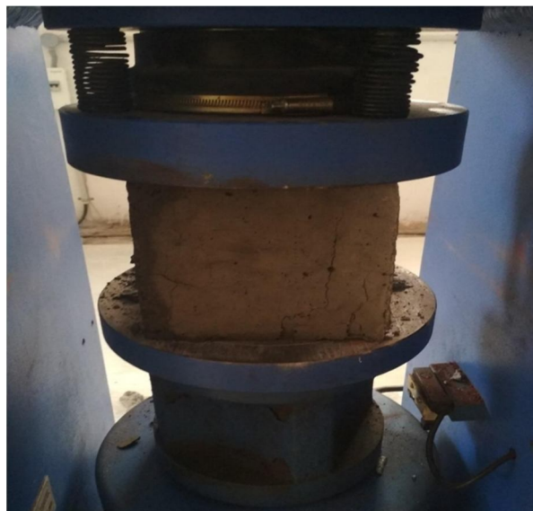
Figure 7. Testing of cube
