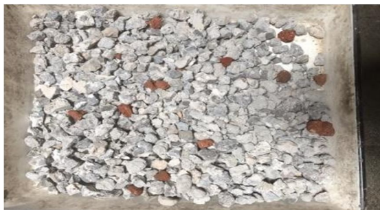
Fig. No. 3.4: Recycled coarse aggregate
