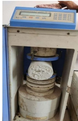
Fig 3: Cylinder under split tensile test
