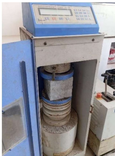
Fig 2: Cube under Compression Test
