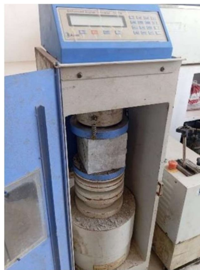
Fig 2: Cube under Compression Test
