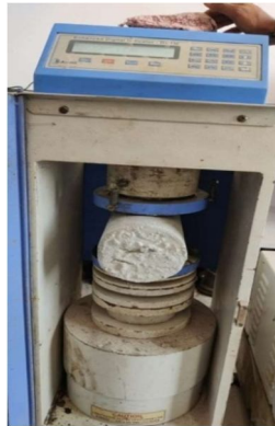
Fig 3: Cylinder under split tensile test
