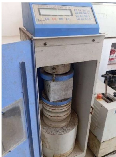
Fig 2: Cube under Compression Test
