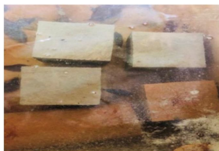
Fig. 3 Specimen Placed in Curing Tank
