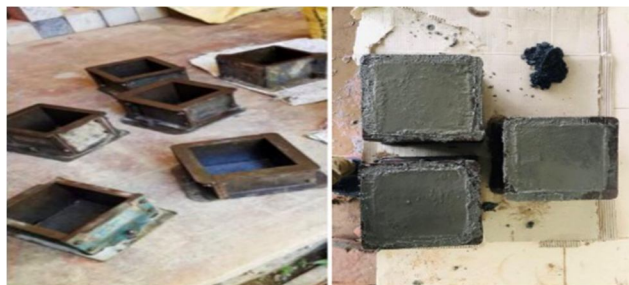
Fig. 2 Casting Mould and Casted Cube
