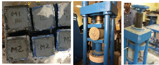
Figure 1: LECA Concrete cubes, split Tensile test and Compressive Strength
