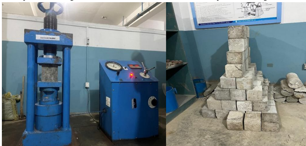
Fig 6: Compressive Strength Test
