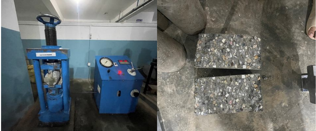
Fig 7: Split Tensile Strength Test
