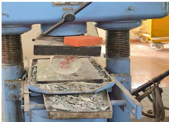
Fig. 3 Split Tensile Strength Test
