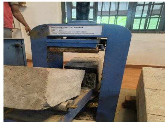
Fig. 4 Flexural Strength Test
