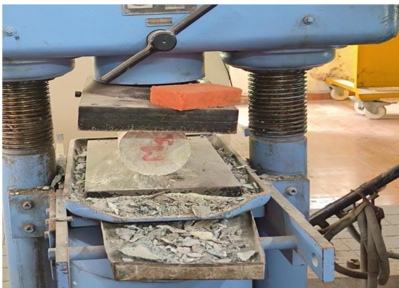
Fig. 3 Split Tensile Strength Test
