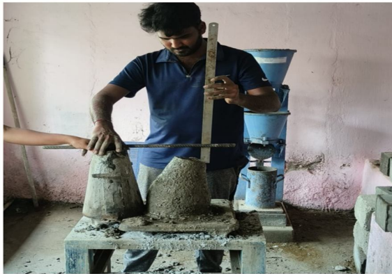
Fig. 1 Slump Cone Test
