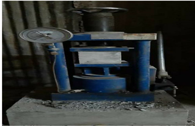
Figure No 4.3:- Concrete Cube under UTM
