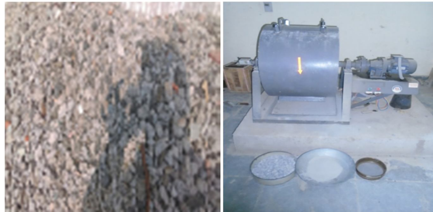
Figure 1 Mechanical Treatment on recycled coarse aggregate
