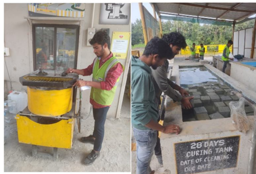
Fig: Mixing of concrete and curing of specimens
