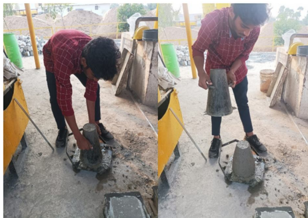
Fig: Slump Monitoring
