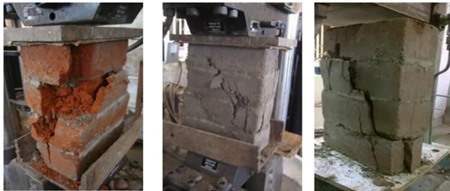
Figure 2: Vertical splitting failure in (a) CB (b) FAB-I and (c) FAB-II prisms
