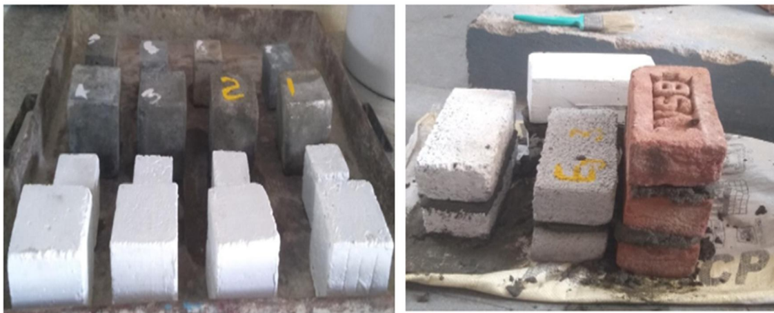
Figure 11: Comparison of bricks without DPC and with DPC and Different Types of Brick Walls
