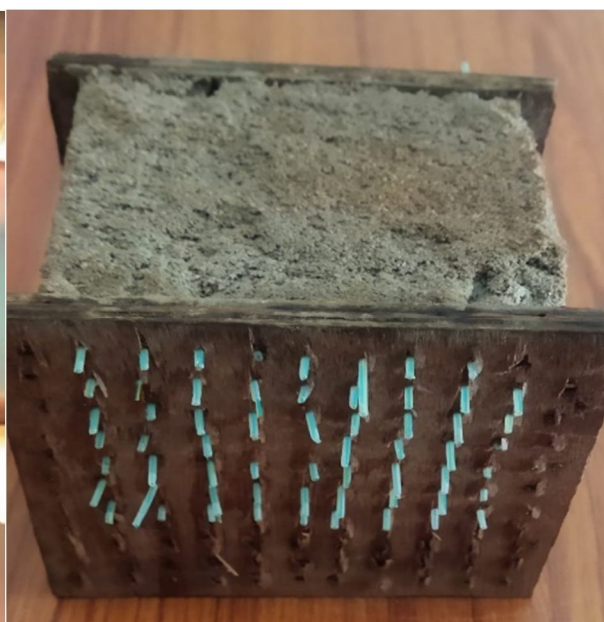
Fig 4 De-moulding of Cube
