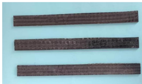
Fig. 4 Specimen section according to ASTM D3039
