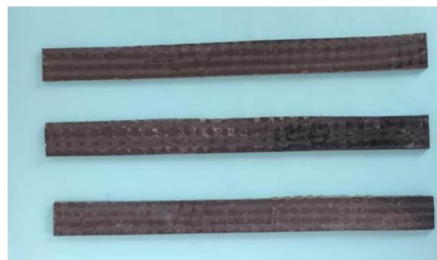
Fig. 4 Specimen section according to ASTM D3039
