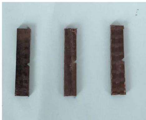
Fig. 7 Specimen section according to ASTM D256
