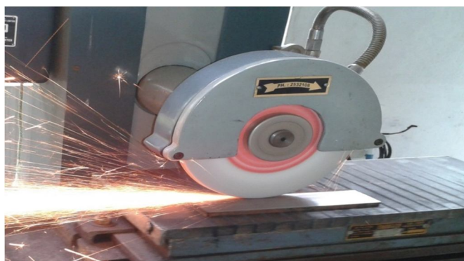
Fig. No. 4.2: Preparation of Plate by Grinding Machine
