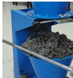
Fig. 8 Compaction Factor Test
