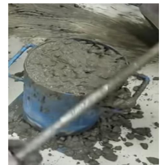
Fig. 8 Compaction Factor Test
