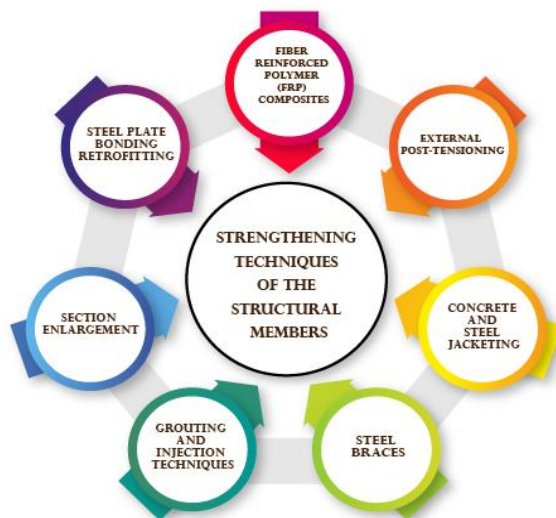
Fig. 1: Strengthening techniques of the structural members
