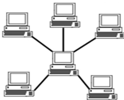
Fig: 6 LAN with STAR topology
