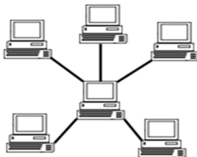
Fig: 6 LAN with STAR topology
