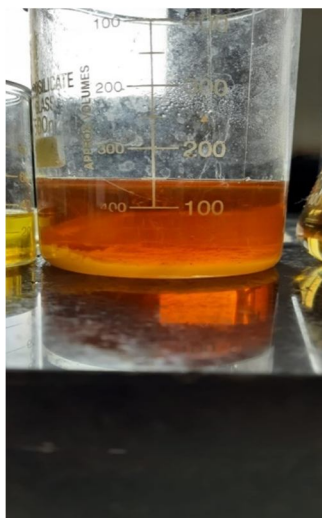
Fig 7: Transesterification mixture after heating
