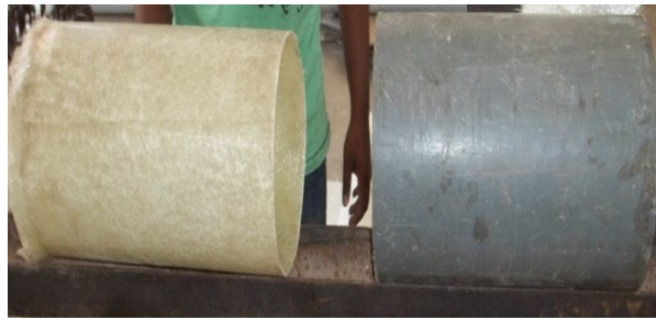
Fig-2 Fabricated glass fiber cylinder
