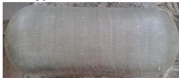
Fig-5: Pressure vessel of 6 layers
