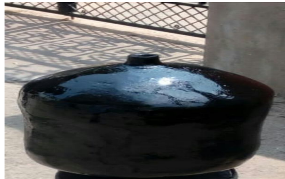
Fig-6: Final fabricated pressure vessel
