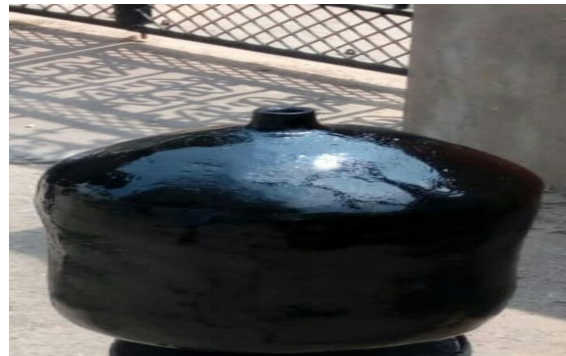
Fig-6: Final fabricated pressure vessel
