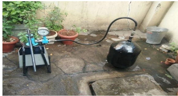
Fig-10: Hydrostatic testing of pressure vessel
