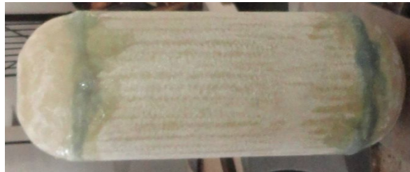
Fig-3: First layer of Pressure vessel
