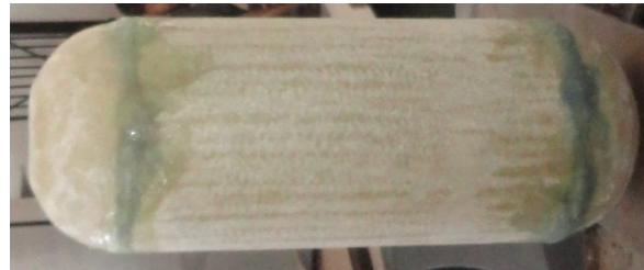
Fig-3: First layer of Pressure vessel
