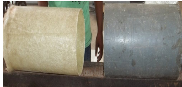
Fig-2 Fabricated glass fiber cylinder
