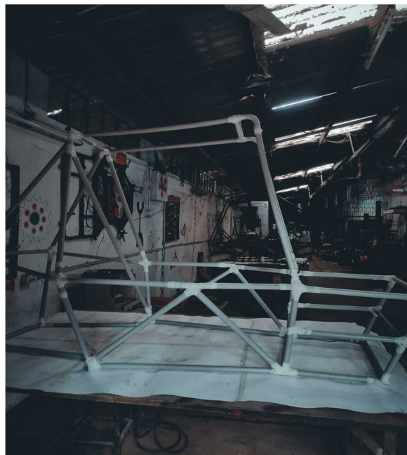
Fig1. plastic model of chassis
