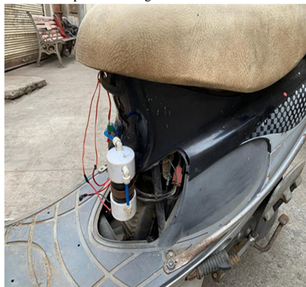
Fig e complete mounting of HHO cell
