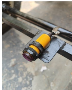
Fig2.2: E18D80NK Proximity Sensor
