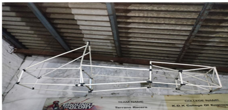
Fig. 2 Prototype of SUPRA kart
