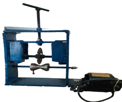
Fig. 6 Assembly of waste cable stripper machine
