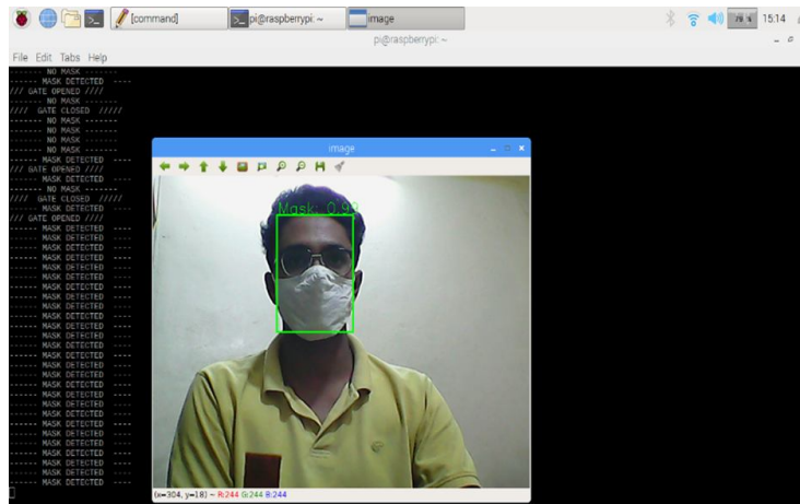
Fig3: Mask detected the system displays “Mask Detected”
