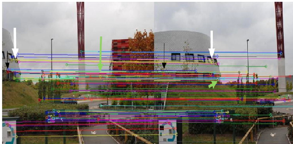
Fig. 2 Mismatched points undetected by Epipolar line filter
