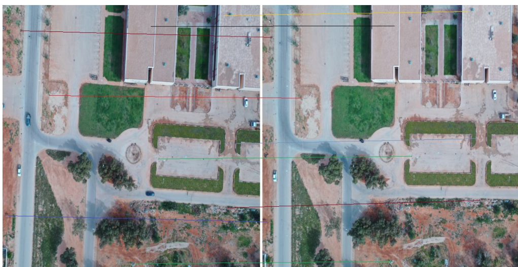
Fig.6 Well-distributed robust automatic matched points
