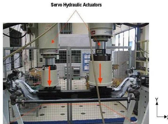
Fig:-Fatigue Loading Testing Setup
