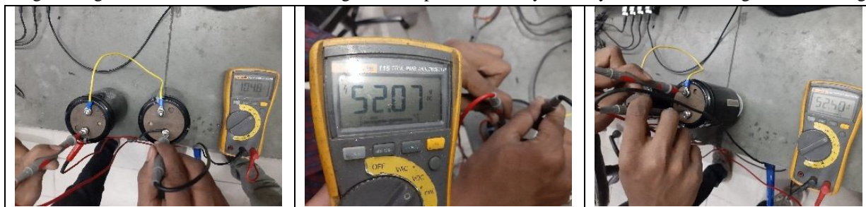
Fig.8 D.C. supply through Capacitor test
