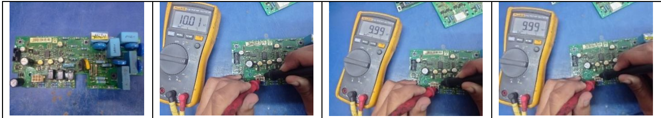
Fig.10 Cold Test of Firing Card
