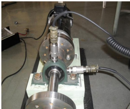
Fig 2 Accelerometer Placed on Bearing, Ch no. 1 of FFT is connected to vertical direction and Ch no 2 of FFT is connected to horizontal direction
