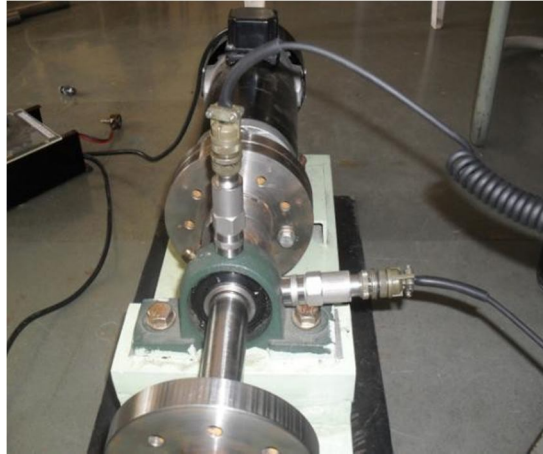
Fig 2 Accelerometer Placed on Bearing, Ch no. 1 of FFT is connected to vertical direction and Ch no 2 of FFT is connected to horizontal direction
