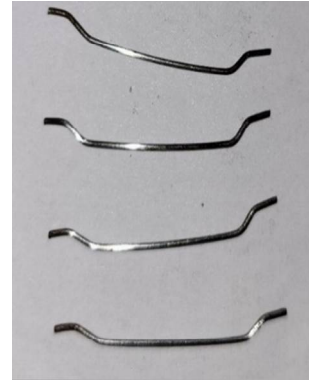
Fig. 15 Hooked end steel fibres
