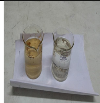
Figure 4: Colour removal sample after root zone system treatment.
