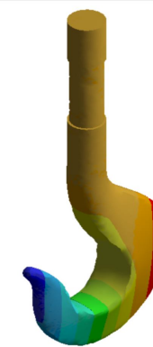
Fig. 8 Deformation – Stainless Steel AISI 1020
