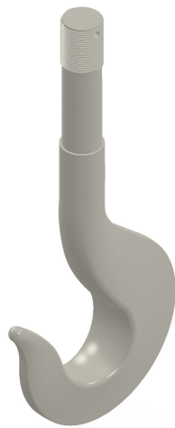
Fig. 1 3D model of the crane hook
