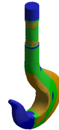
Fig. 10 Safety factor – Stainless Steel AISI 1020
