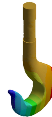
Fig. 8 Deformation – Stainless Steel AISI 1020
