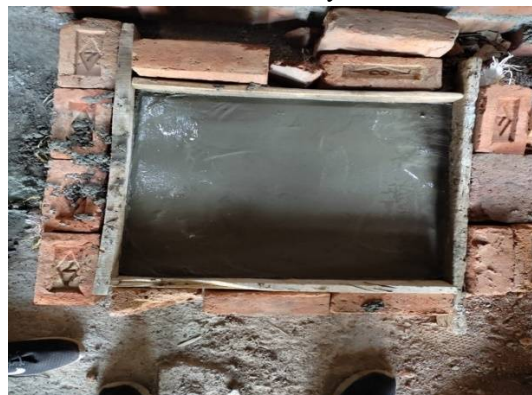
Fig. 2: Slab cube casted
