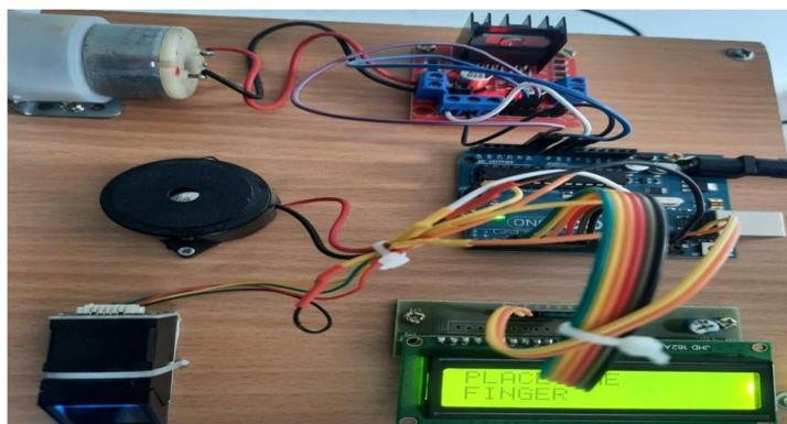
Figure 7. figure represents output message on LCD
