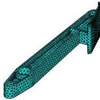
Fig. 4. Tetrahedral mesh of max 0.005 m and min 0.003 m size with a growth gradient of 1.6 in MATLAB
