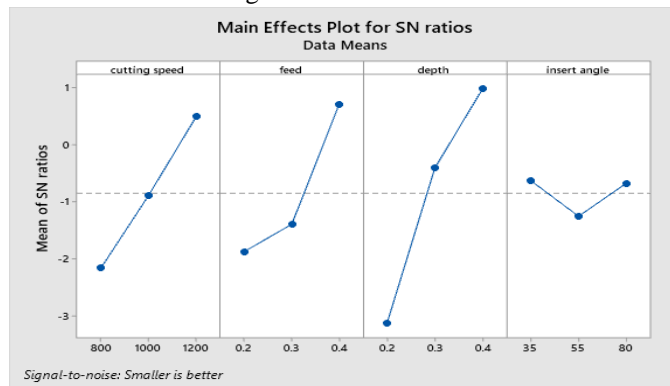
Fig. 14 Main effects plot for S/N ratio of machining time
