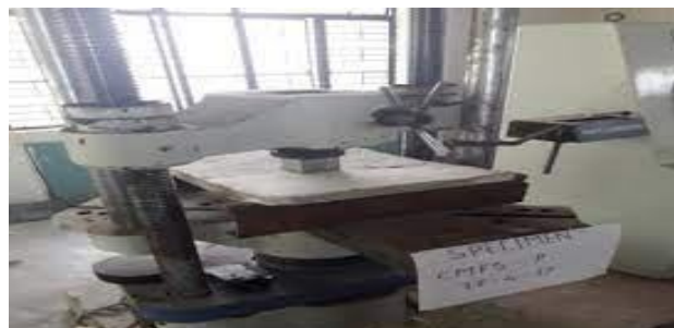
Flexural Strength Test on Beam
