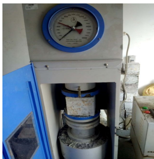
Compression Test on Cube
