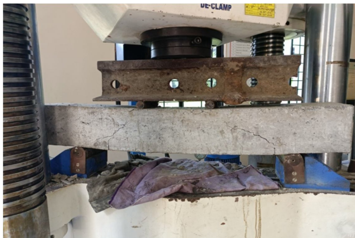
Figure 2 – Test Setup for Flexural test
