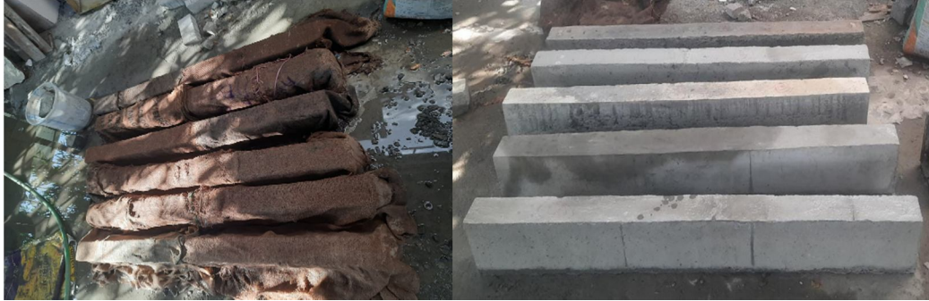
Fig. 1 Casting and Curing of Beams
