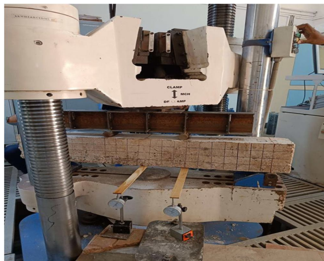
Figure 15 Flexural Test for 5% Replacement Beam
