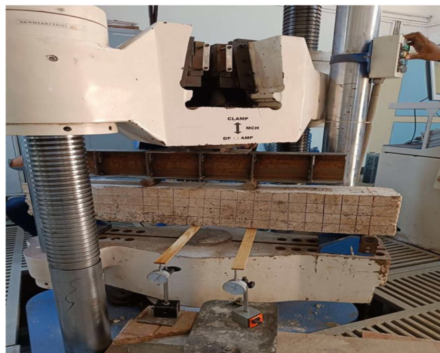
Figure 15 Flexural Test for 5% Replacement Beam
