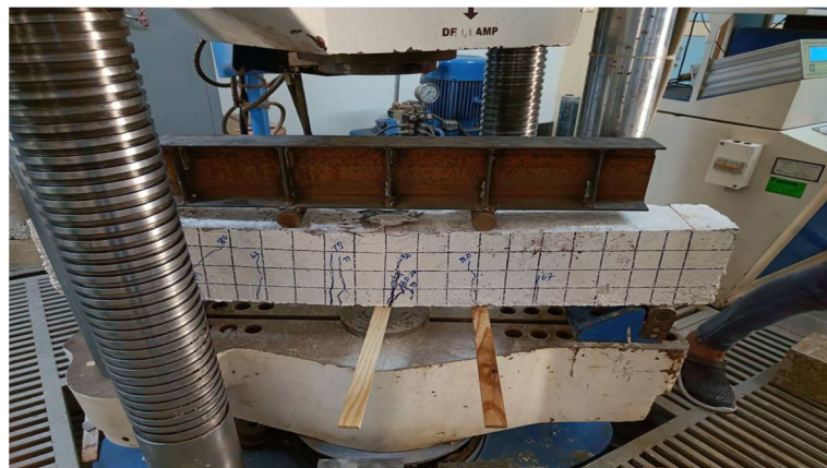
Figure 18 Flexural Test of 10% Replacement Beam
