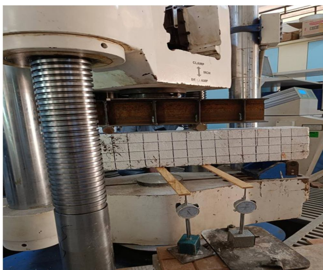
Figure 20 Flexural Test of 15% Replacement Beam
