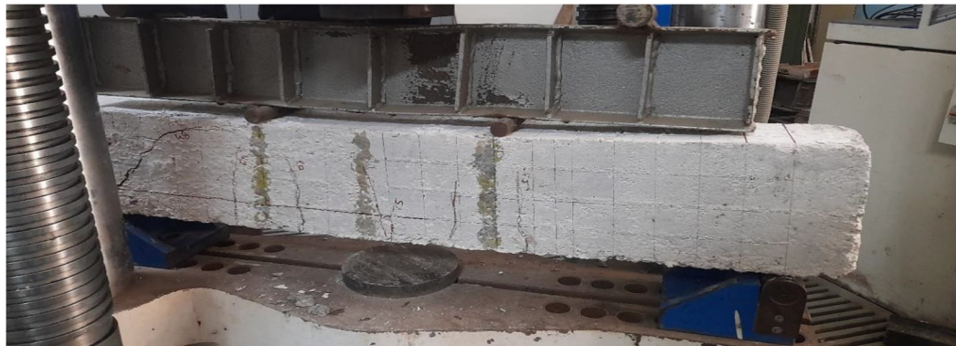
Figure 13 Testing of Normal Beam
