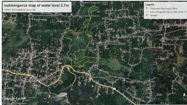
Fig.4 Flood inundation map of Pariyaram by google earth at water level 2.7m
