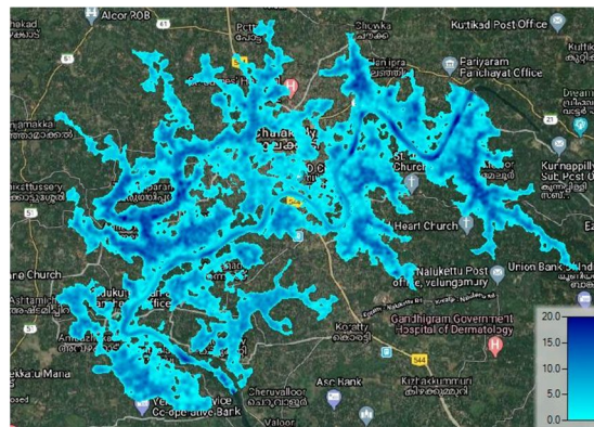
Fig. 3 Inundation depth for flood prone areas
