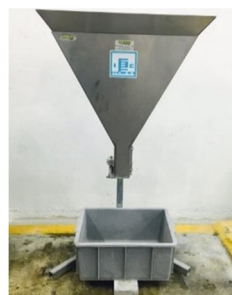
Fig. 3: V-Funnel test apparatus
