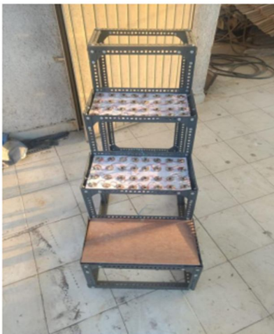
Figure 2: Arrangement of wooden plates over the sensors and movable springs
