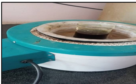
Figure 4: Heating with Heating Mantle
