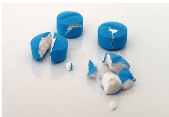
Fig 14: defect in tablet
