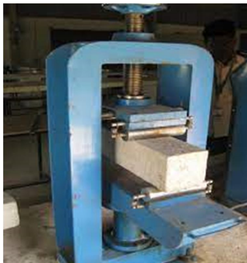
Fig. 7 Flexure strength test
