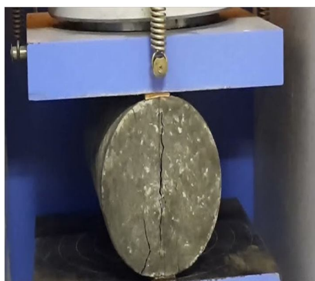
Fig. 5 Split tensile strength
