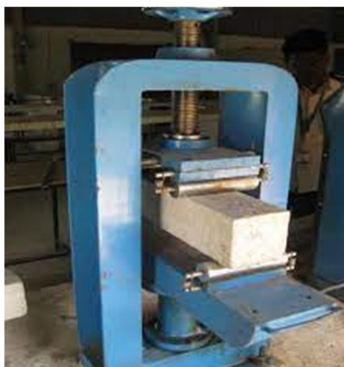
Fig. 7 Flexure strength test
