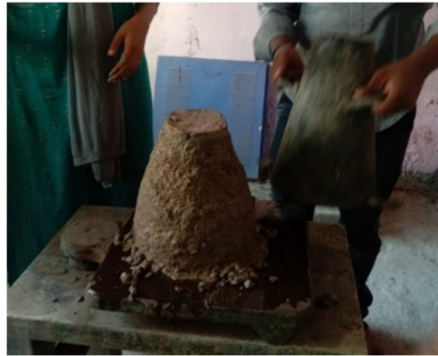
Fig. 1 Slump Cone Test
