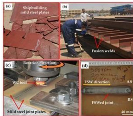
Fig.22-Figure depicts mild steel plates used in shipbuilding (Figure 1a), traditional fusion welding in shipbuilding (Figure 1b), the FSW process of mild steel plates (Figure 1c), and a top view of an FSWed butt joint (Figure 1d) (Figure 1d)
